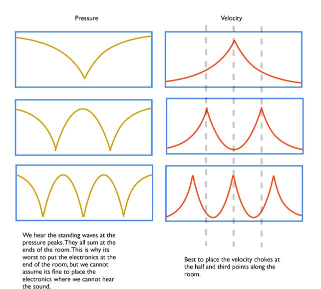
The micro-hole panels are very efficient at lowering the velocity component. Drag increases with the square of velocity. Because the standing waves buid up with resonant tendencies we will get an uneven velocity profile within the room.
