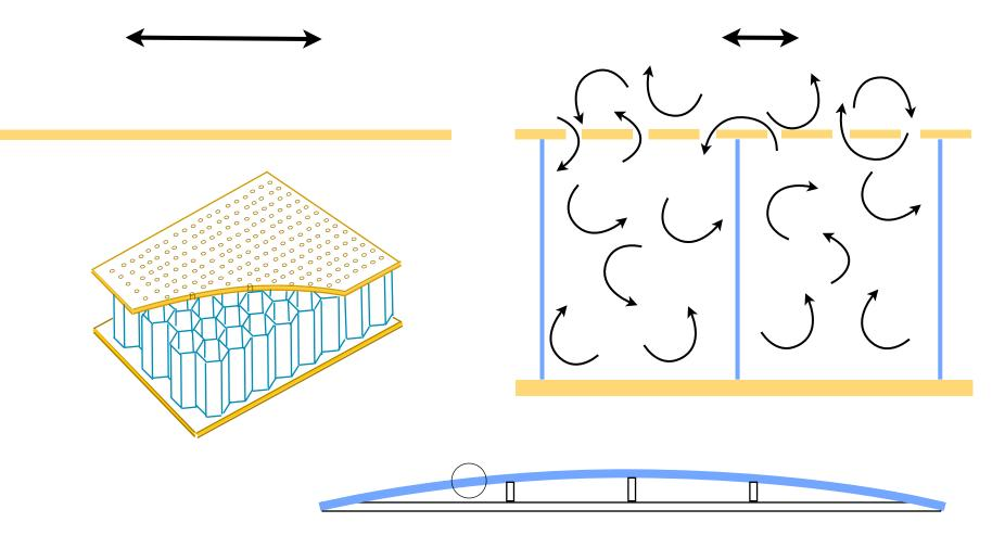
This is how the micro-hole acoustic panels are constructed internally. They work in a completely different way to foam, and are far more effective than foam, therefore requiring less surface area in a room to have a great effect.
