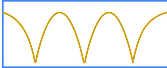
We hear the standing waves at the pressure peaks. They all sum at the ends of the room. This is why it's worst to put the electronics at the end of the room, but we cannot assume it's fine to place the electronics where we cannot hear the sound.
