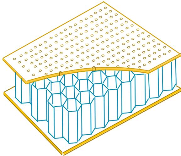
In the vicinity of the micro-hole surface, as the velocity component builds, there is a corresponding rise in aerodynamic drag, absorbing energy from the velocity part of the wave.
