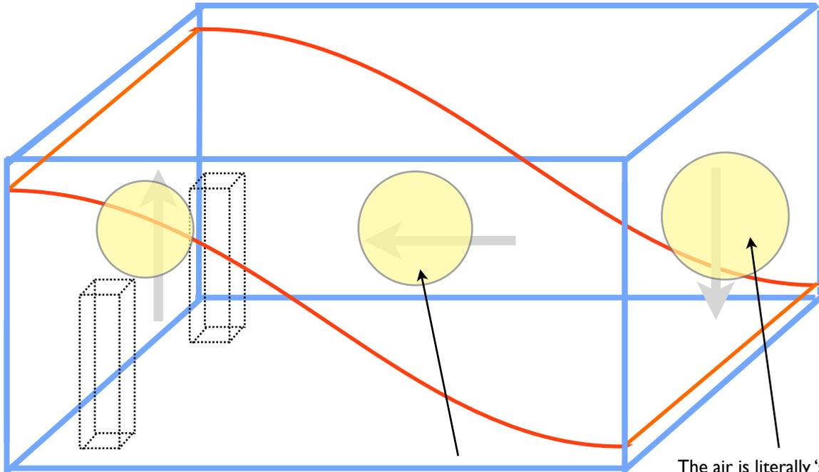
There is no pressure change here - so we don't hear any sound. The wave is purely in its velocity mode. The air's energy is in the form of momentum here.
